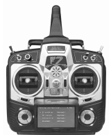
3. Pull down the throttle stick and throttle trim of transmitter to the lowest position, and then move the elevator trim, aileron trim, and rudder trim at the neutral positions, respectively.
