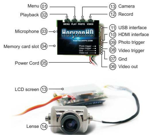
**horyzonhd V3 has auto-on function, no power button is necessary.**
